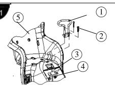
Insert the handgrip (1) into the square hole of the Baby carrier (5)
