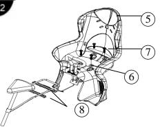
Position the baby carrier (5) on the carrier and at the same time, put the Iorn Sheet (8) under the carrier. Make sure to set the correct position of the baby carrier Before tightening the screws (6) (7).
