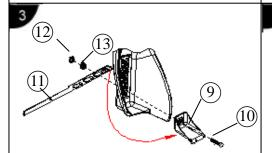
Install the footrest on the baby carrier (5). Make the foot strap (11) go through the footrest side
